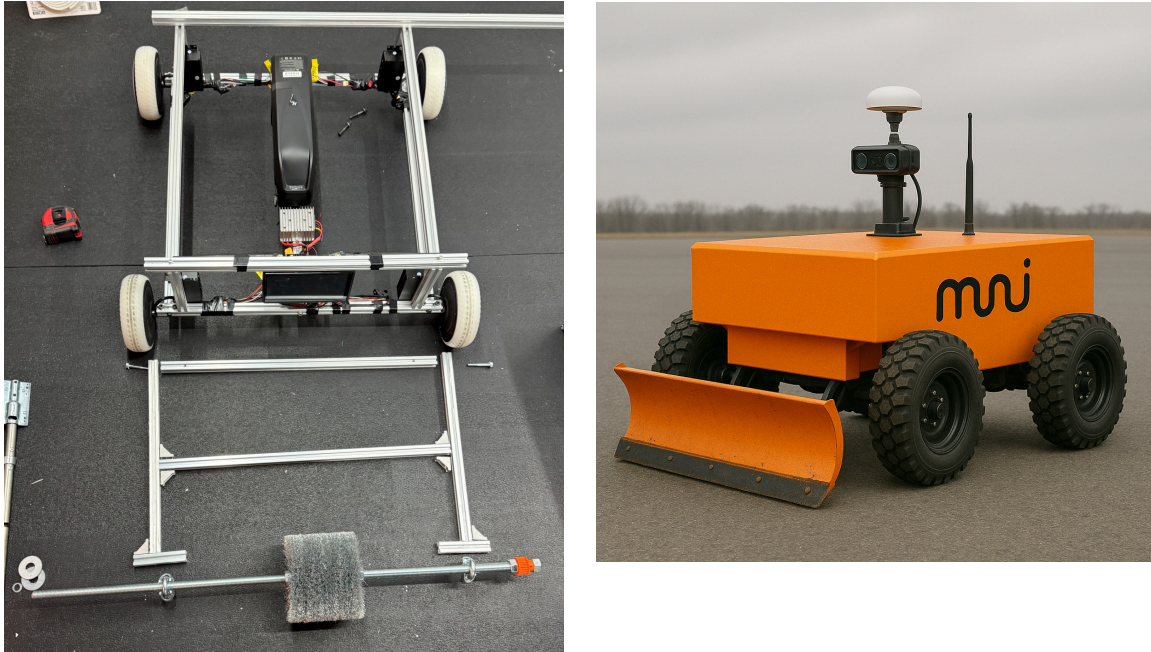
Figure 9: Left: BVR0 disassembled for maintenance: aluminum extrusion frame, hoverboard hub motors, e-bike battery, and modular plow attachment. All components replaceable with hand tools in under 30 minutes, with parts generally available from big box stores. Right: BVR1 (rendering), precision-engineered production unit shipping to pilot customers, featuring enclosed weatherproof chassis, integrated plow, RTK GPS, and stereo vision.
