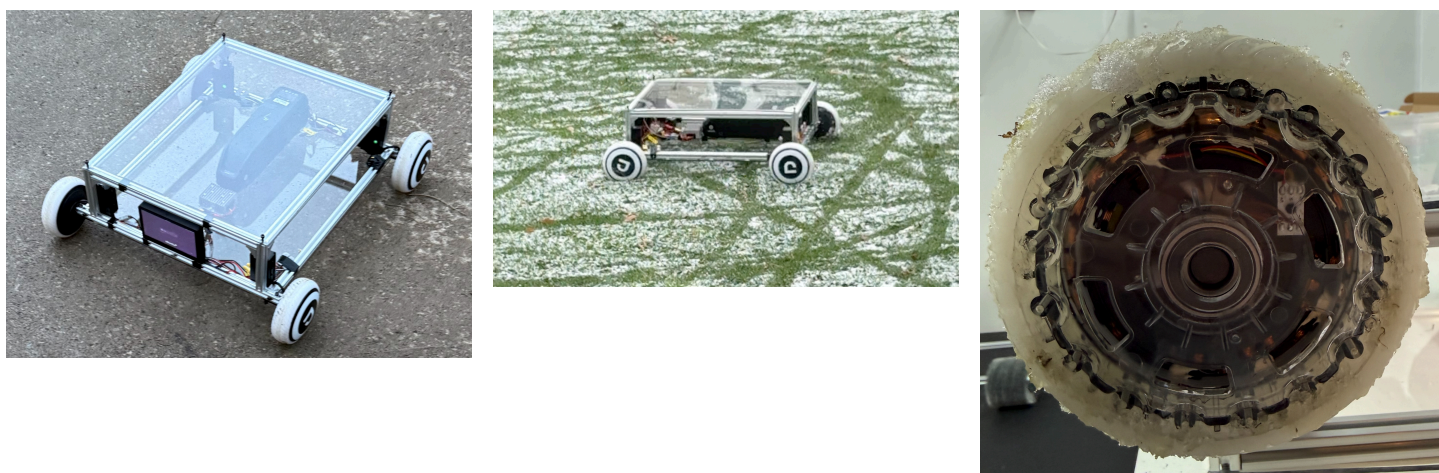
Figure 8: BVR0 engineering prototype: ultra-low-cost, field-repairable. Pavement testing (left), mid-drift maneuver on grass (center), hoverboard hub motor after snow operation showing acceptable winter traction (right)
