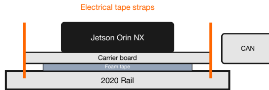
Figure 18: Jetson mounted with foam tape and electrical tape straps.
