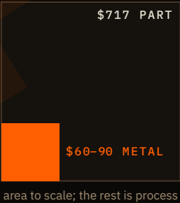
FIG 13 The idiot index. Cost over raw-material cost, for the manufactured parts of rana-100 (housing, magnetic steel, gear blanks) in Figure 12. Estimates.
